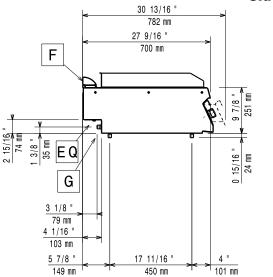
EQ = Equipotential screwG = Gas connection
